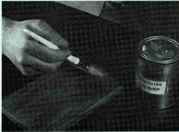
Figure 7. "Flowing" the brushing lacquer on the wood sample panel.
