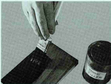
Figure 5. Applying a wood filler over the washcoat.
