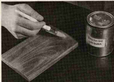
Figure 7. "Flowing" the brushing lacquer on the wood sample panel.
