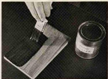
Figure 5. Applying a wood filler over the wash-coat.
