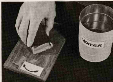
Figure 8. Rubbing the finished surface using wet/dry sandpaper and water. Note the circular motion.
