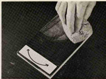
Figure 6 Wiping the wood filler using a rotary motion.
