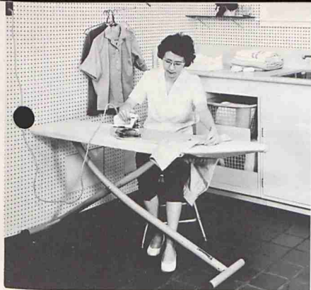
Garment hook and hangers are within easy reach. The electric outlet is high enough and far enough forward of the ironing board to provide a natural cord holder.
