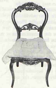
Fig. 59 —Burlap is slip tacked over the padding before stitching the hard roll around seat edge.
