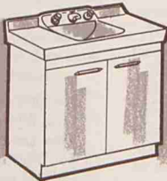
Lavatory-counter top set on cabinet.
