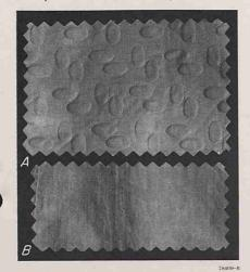
FIGURE 38.—Embossed patterns on cotton: A, Before being worn; B, flattened with wear.
