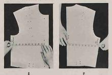
E. Bust front.—Measure between center front and side-seam lines, 2 inches below armhole seam line.
