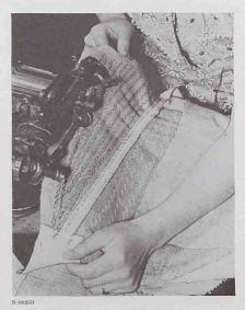
Machine stitching replaces hand shaping and stitching in medium- and low-grade suits. The lower the grade, the less stitching.
