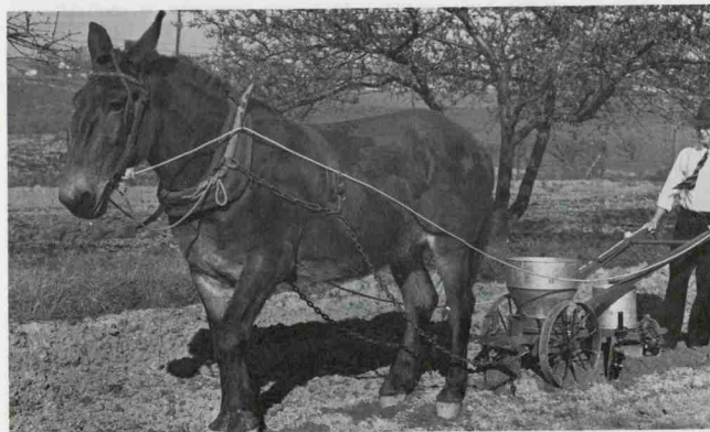
Fig. 10. The second research project was a one-row planter with side placement of the fertilizer. Dean of Agriculture I.O. Schaub is shown above operating the first prototype.
