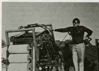
E. C.F. Abrams, Jr. examines side delivery part of sweet potato harvester he is working on.
