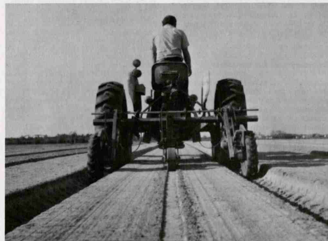
Fig. 32. Precision bedding and planting of cucumber seed is necessary for a successful mechanical harvester—a systems approach.
