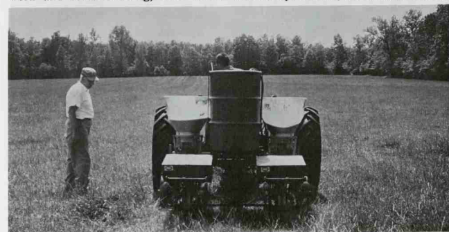
Fig. 7. J.C. Ferguson stands beside the no-till planter he adapted for moisture conservation situations such as the pasture land shown.
