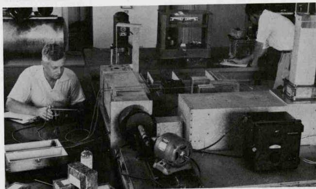
Fig. 14. The department's first model experimentation in the laboratory was with drying hay in the bale. Note the miniature bales in the foreground. J.W. Weaver, Jr. is on the left and S.H. Usry is on the right.
