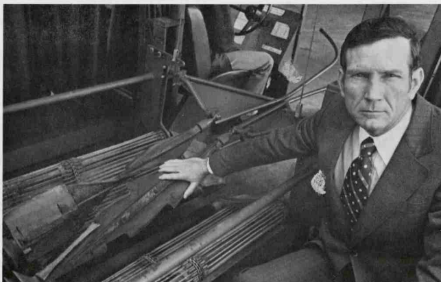
Fig. 23. Charles W. Suggs earned the first Ph.D. in Agricultural Engineering in 1959. He is shown here with the world's first tobacco leaf harvester which he helped develop. His hand rests on the unique leaf stripper widely used in commercial harvesters today.
