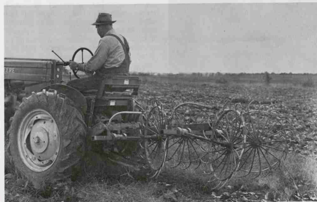
A. The world's first finger-wheel rake is used on sweet potato vines.
