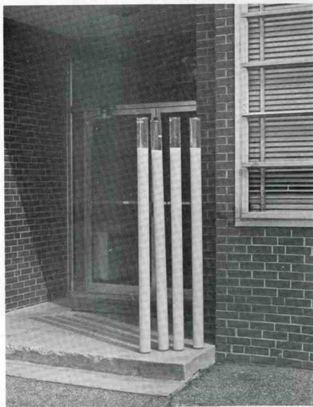
Fig. 35. Experimental Clear Cylindrical Latent Heat Storage Elements.
