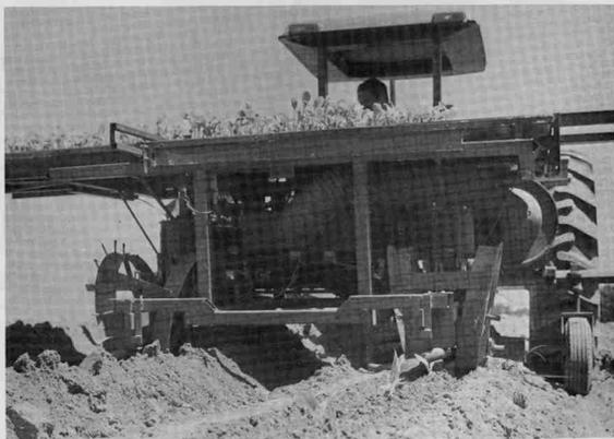
Fig. 28. Field Transplanting of Solar Barn Grown Tobacco Transplants Using the Two-Row Fully Automatic Transplanter.
