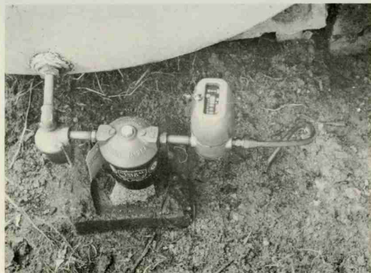
Figure 3. Flow meters for gas (left) and oil (right) were installed in the fuel supply line of each test barn in the 1964 tests.
