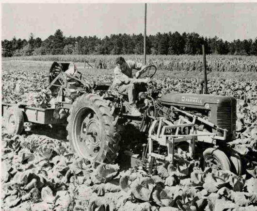
Figure 8. View of 1963 model experimental cabbage harvester operating in the field.
