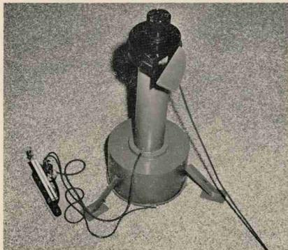
Fig. 2 Experimental device for measuring air-flow rate
