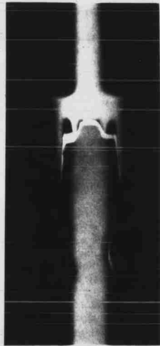
White areas on radiograph show where solder was used on sword.
