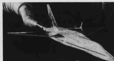
⑤ AERODYNAMICS LABORATORY facilities include several wind tunnels—ranging from subsonic through hypersonic at Mach 10—which are used to determine and improve static stability, control and heat transfer characteristics of helicopters, VTOL's, supersonic aircraft, missiles, etc. Air flow studies also involve bomb design, bridge structures, aircraft turbulence when approaching carriers, and other government and private problems.
