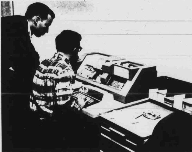
This is one of the card punch machines in the Computing Center in the basement of Nelson that is maintained by the Center and made available for student use on projects. The primary use is for students in CSC courses, but other students use it also.
