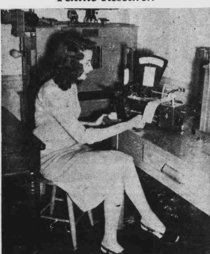
Martha Wallace, laboratory technician in the School of Textiles at N. C. State College, is pictured as she operates the roving tester, a device for determining the tension, evenness, and twist of the fiber in the process of yarn manufacturing. The instrument, along with many other complex pieces of machinery, have been contributed to the College's School of Textiles by the North Carolina Textile Foundation, making the school second to none in the world from the standpoint of its research and educational programs.
