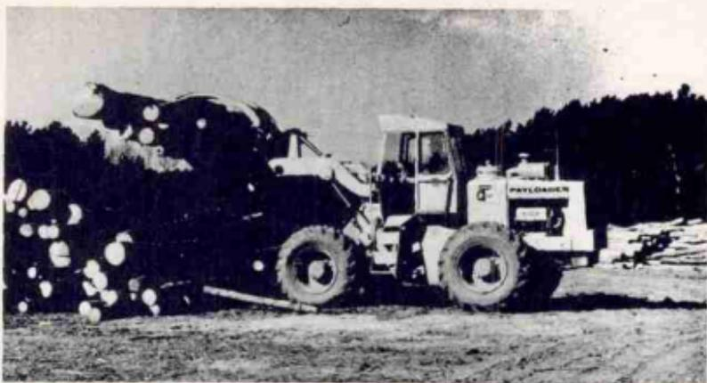
Hough Model H-60B PAYLOADER with Grapples loading logs.
