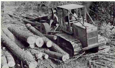
International TD-9B Crawler Tractor snaking logs in eastern North Carolina.
