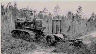
International TD-9 Crawler Tractor equipped with Hester Fire Line Plow.
