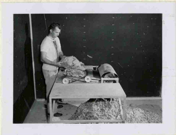
Figure 4. Tobacco leaves were shredded to uniform width by this electrically powered shredder using a reel-type blade.
