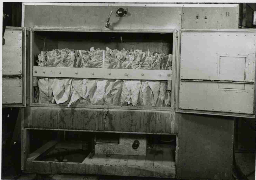
Figure 2. Climatic chambers of this type, having sensitive electronic temperature controls and air recirculation dampers, improved the quality of cure.
