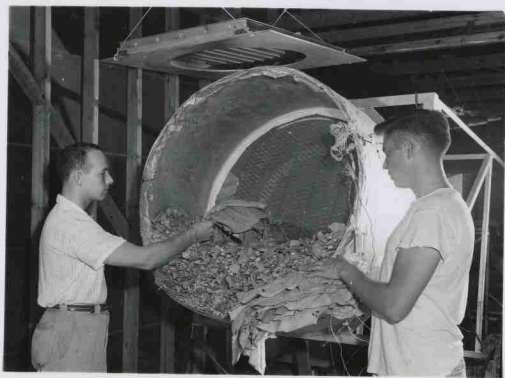
Figure 5. Intact tobacco was placed by the handful into the bulk-curing chamber. After filling, the chamber was placed in its normal vertical position for the curing process.
