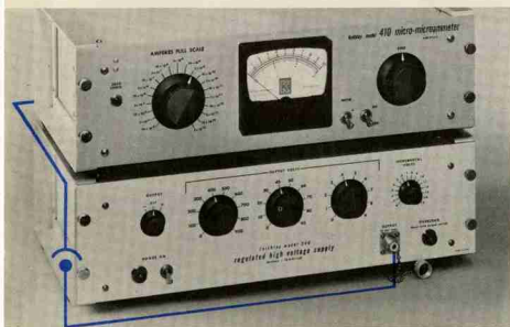
FIGURE 4. The Keithley 410 Micro-microammeter measuring photocell current, with excitation voltage furnished by the 240 Supply. The broad range of output voltages available with the 240 makes it an ideal choice for testing the sensitivity and linearity of photocells, photomultiplier tubes, and ionization chambers.
