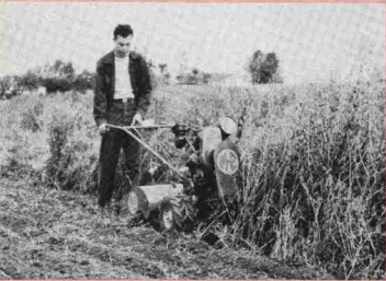
Bolens M-E Rotary Tiller shown turning under heavy vegetation. Every model does an excellent job of soil-preparation and soil-building.
