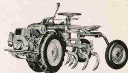
Bolens Ridemaster Tractor Front wheel drive, 6 h.p. engine.
