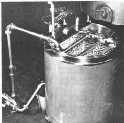
Dairy Foundation funds helped develop equipment such as this, made available to the dairy industry in 1948, which removed objectionable off-flavors from milk.
