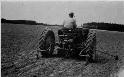
A two-row, tractor-mounted planter, with fertilizer attachments for band placement and row marker. This machine can plant 2 acres per hour.
