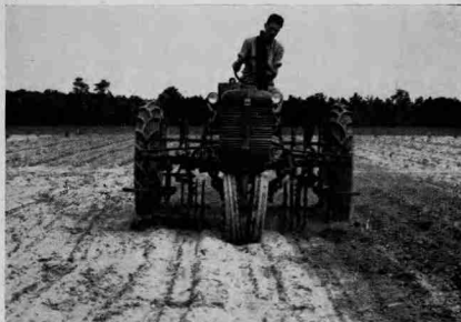
A two-row tractor, equipped with rotary hoe attachments, cultivating small cotton at 5 m.p.h.
