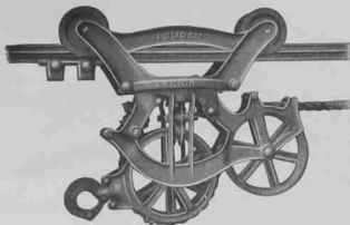
Showing Swinging Fork Pulley Loads can be dragged over beams or other obstructions without endangering carrier.
