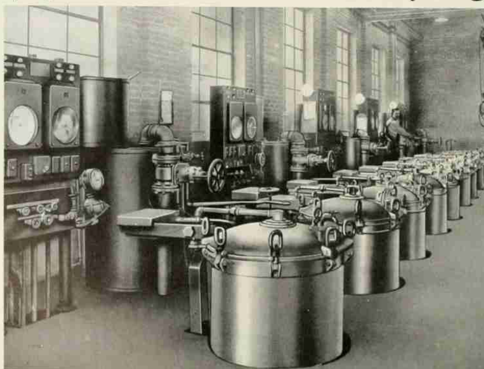
Recent Installation of Combination Beam and Package Dyeing Machines
