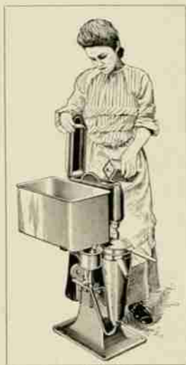
OILING THE DAIRY TUBULAR
