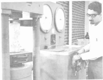
Concrete cylinder strength is tested in civil engineering lab.
