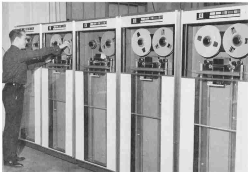
Computing Center—The IBM 1410 Tape System provides the computing facility for faculty and students in research and instruction. Two IBM 1620's and a LINC III furnish additional computing capabilities for some departments.
