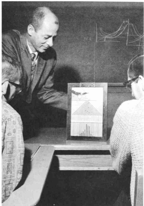
EXPERIMENTAL STATISTICS—The laws of probability are demonstrated by dropping steel balls in a Quincunx.
